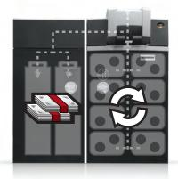
The **transfer** of notes from the recycling area to the deposit one is **totally automated** and secured. No note in the recycling part is accessible during the transition. In order to provide further security, the CM24B **safe is divided into two** different parts, one for recycling and the other for deposit. Every safe is opened by different electronic locks allowing different individuals to have access to the machine in total security.
